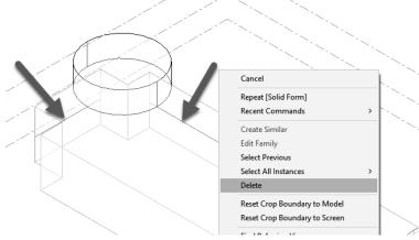
Select the two lines used to locate the circle sketch.
