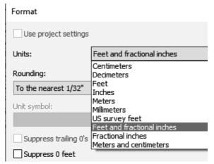
Left click the Length button, then select the desired units from the drop-down list. Double click **East** under Elevations.
