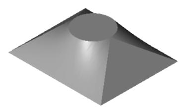
2) Make the shape shown using a Blend. The base is a rectangle and the top is a circle located at the center of the rectangle.
