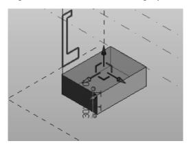
You can use the triad on the top of the extrude to extend the shape in any of the three directions.
