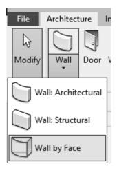
This tool can be used to place walls on non-horizontal faces of a mass instance or a generic model.
