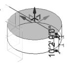
A preview of the extrusion will appear with the temporary dimension. You can edit the temporary dimension to modify the height of the extrusion.
