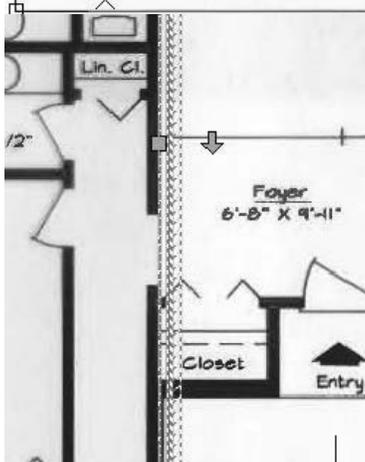
Flip the wall orientation so the wall exterior is on the outside of the building.
