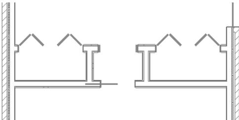
Place the arched opening in the wall between the closets in the Master Bedroom. Center it on the wall.
