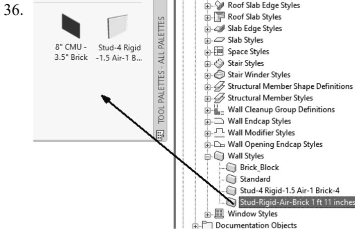
Drag and drop the new wall style onto the Walls tool palette.
