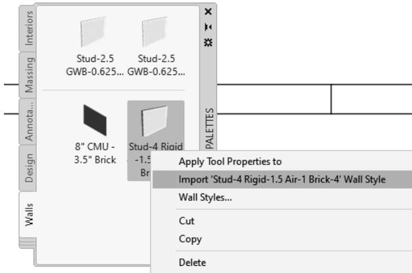
Right click on the **Stud-4 Rigid-1.5 Air-1 Brick-4** wall style and select **Import Stud-4 Rigid-1.5 Air-1 Brick-4** wall style.
