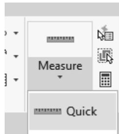
Use the Quick Measure tool to check the offset distance to ensure the two walls are 15' apart from inside finish face to inside finish face.
