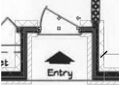
Select the side of the wall that will be used for the door swing and place the entry door.
