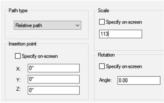
Uncheck the insertion point to insert the image at **0, 0, 0**.
