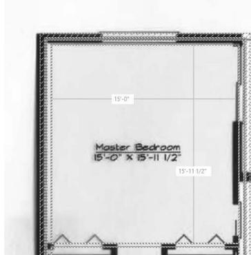
**MOVE** the top horizontal wall as needed to get the correct dimensions.
