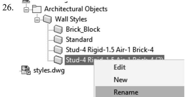
Highlight the copy of the **Stud-4 Rigid-1.5 Air-1 Brick-4** wall style.
