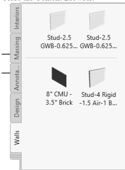
Place the wall style in the area used by exterior wall styles.
