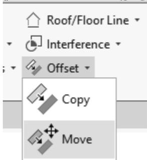
Use the **OFFSET** tool to move the interior walls to the correct position.
