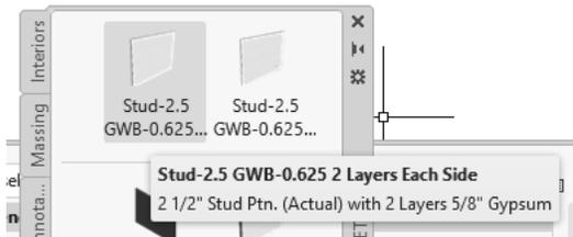
Locate the **Stud-2.5 GWB-0.625-2 Layers Each Side** Wall Style on the Walls tool palette.
