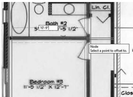
Move the mouse slightly to the right. Type **10'-9\"** as the offset distance.
