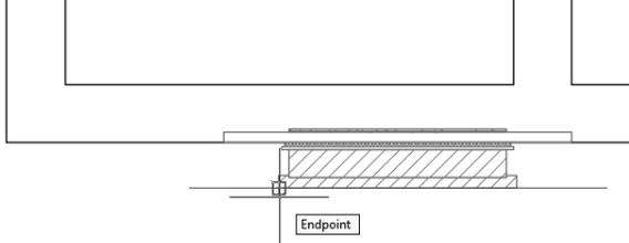
Move the cursor over the wall until the face of the component you want is highlighted with a red line, and click once.
