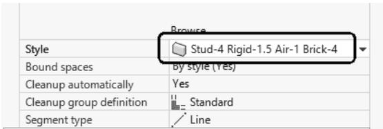
Select the **Stud-4 Rigid-1.5 Air-1 Brick-4** wall style from the Style drop-down list on the Properties palette.
