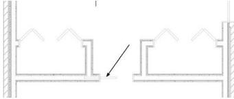
Center the pocket door on the lower horizontal wall between the Master Bedroom closets.
