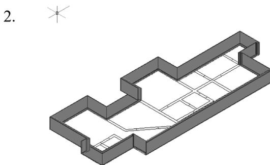
To join the walls together, use FILLET with an R value of 0.
