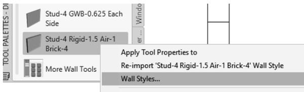
Right click on the **Stud-4 Rigid-1.5 Air-1 Brick-4** wall style and select **Wall Styles**.
