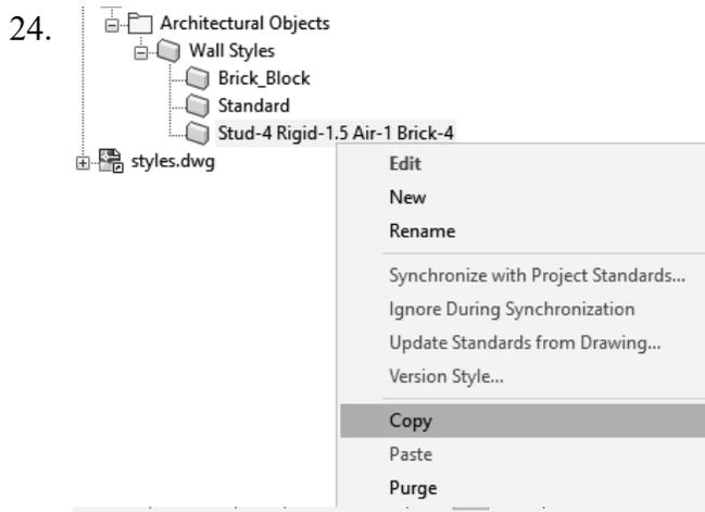
Highlight the **Stud-4 Rigid-1.5 Air-1 Brick-4** wall style.
