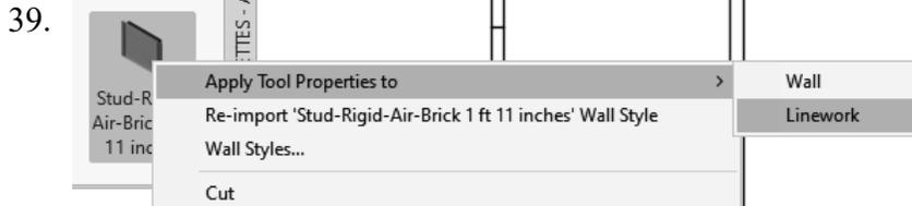
Right click on the **Stud-Rigid-Air-Brick-1 ft 11 inches** wall style and select **Apply Tool Properties to** → **Linework**.
