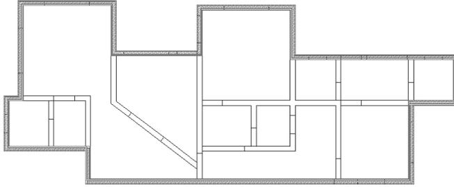
In the plan view, the exterior walls should form a closed figure.
