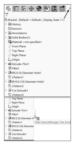
The Sensors tool located in the FeatureManager monitors selected properties in a part or assembly and alerts you when values deviate from the specified limits. There are five sensor types: Simulation Data, Mass properties, Dimensions, Measurement and Costing Data.
