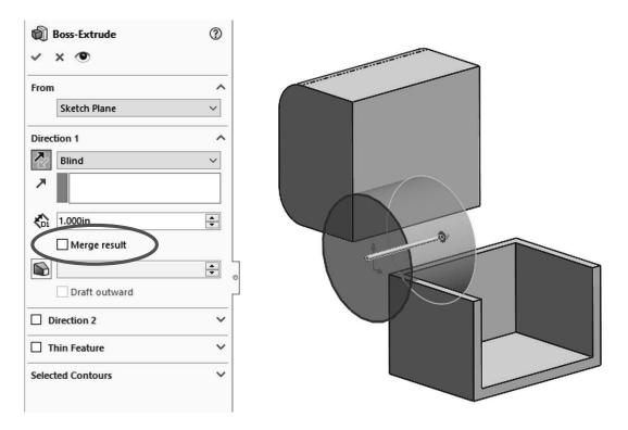
**1.7.** - After adding this extrusion we have three different bodies in our part. See how the different bodies' edges intersect each other. If the "Merge result" option had been checked, we would not see the overlapping edges as they would be merged into a single body.
