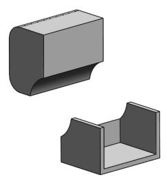
**1.10. -** Edit the "*Cut-Extrude1*" feature, turn the "Auto-select" option OFF in the "**Feature Scope**," and select the top body only. Click **OK** to finish. Now we are only cutting into the top solid, even if the cut overlaps the lower body.
