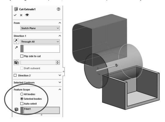
And just as with the features that add material, this technique works the same way with all the features that remove material including revolved cut, sweep cut, loft cut, etc.
