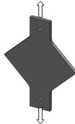
Figure 37 - Model subject to “equal” but opposite forces.
