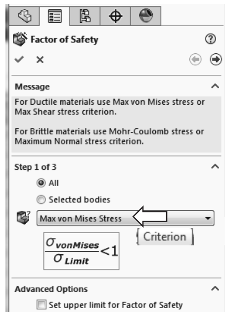
Figure 28 – The failure criterion is selected in Step 1 of 3 of the Factor of Safety dialogue box.
