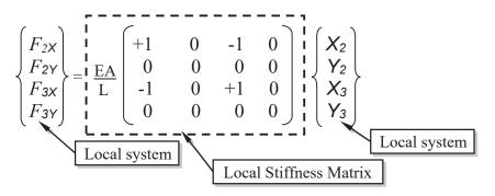
Using the equations we derived in the previous sections, the GLOBAL system equation for *Element B* is:
