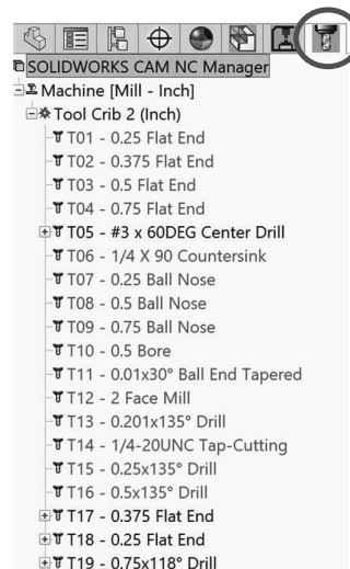
Figure 1.13 SOLIDWORKS CAM tools tree tab
