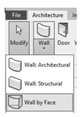
This tool can be used to place walls on non-horizontal faces of a mass instance or a generic model.
