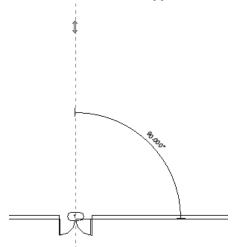
Select the center of the door as the start point of the mirror axis.
