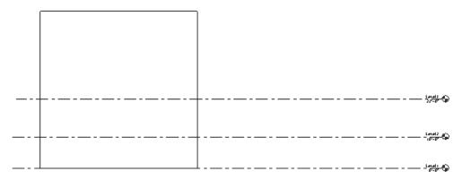
To adjust the horizontal position of the level lines, simply select the line and use the grip to extend or shorten it.
