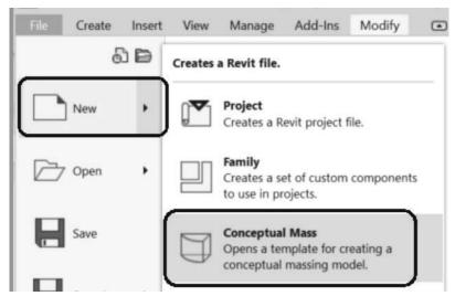
Create an extrude, revolve, sweep and blend using New→Conceptual Mass from the Applications menu.
