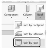
Select the Roof by Face tool on the Build panel.
