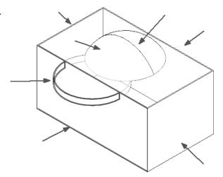
Select the four sides of the box, the outside arc of the cylinder and the two sides of the dome to place walls.
