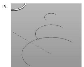
Our final shape will be a BLEND or LOFT. A blend is created using two or more open or closed sketches. Each sketch must be placed on a different reference plane or level.
