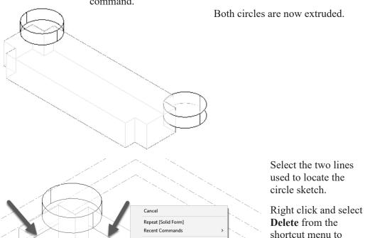
You can also click the Delete key on the keyboard or use the Delete tool on the Modify panel.
