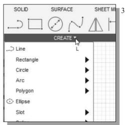
3. Click and press on the **Sketch** tab in the main *Ribbon* area to display the additional available sketching tools as shown. Also note the **Sketch Palette** panel is also activated with a varity of sketching options.
