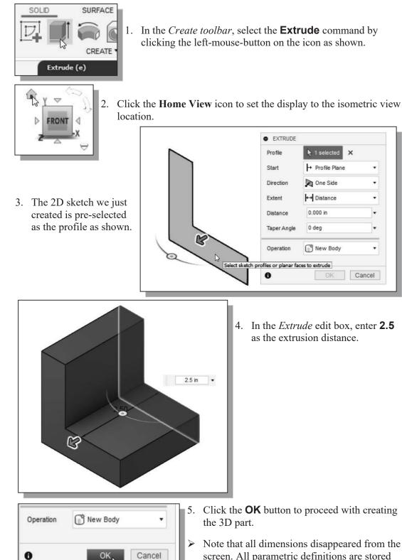
> Note that all dimensions disappeared from the screen. All parametric definitions are stored in the database and can be re-displayed.
