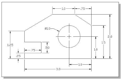
2. Spacer Plate (Thickness: .125)
