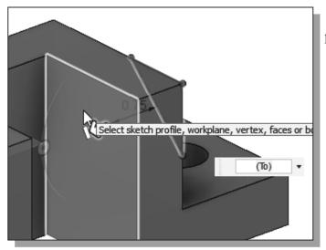
12. On your own, use the dynamic rotate function and select the back surface as shown.
