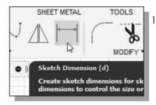
In the sketch toolbar, select the Sketch Dimension command as shown. The Sketch Dimension command is generally known as Smart Dimensioning in parametric modeling. 2. The message "Select Geometry to Dimension" is displayed in the Status Bar area at the bottom of the Fusion 360 window. Select the bottom horizontal line by left-clicking once on the line.
