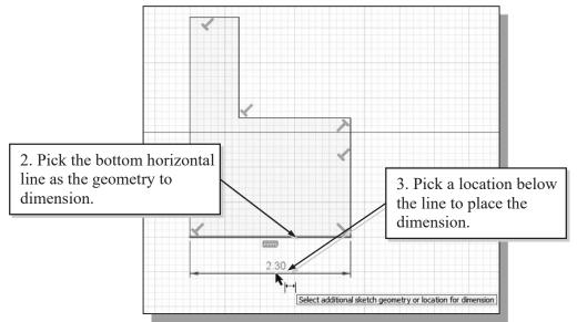
3. Move the graphics cursor below the selected line and left-click to place the dimension. (Note that the value displayed on your screen might be different than what is shown in the figure above.)
