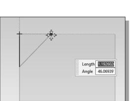
5. Place the second point aligned to and to the right of the sketch origin as shown.
