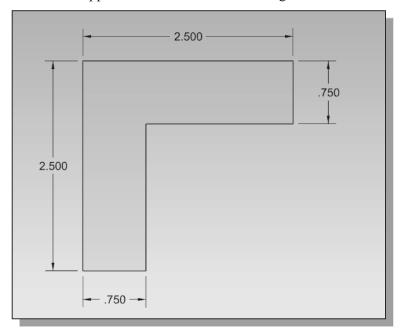
❖ In Siemens NX, this **Rapid Dimension** command is also known as the **Smart Dimension** command; dimensions are created based on the selection of the types and orientations of objects. You might want to read through this section again and consider the powerful implication of this command. Also consider this question: How would you create an *Angle dimension* using the *Rapid Dimension* command?
