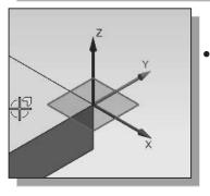
Note that the sketch plane is aligned to the selected face. Siemens NX automatically establishes a Work-Coordinate-System (WCS) and records its location with respect to the part on which it was created. 3. Select the **Circle** command by clicking once with the **left-mouse-button (MB1)** on the icon in the *Sketch Curve* toolbar.
