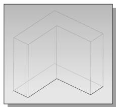
**❖** Wireframe with Dim Edges
