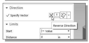
11. In the Direction option box, use the **Reverse Direction** icon to toggle the extrusion direction so that the extrusion cut through the bottom section of the model.
