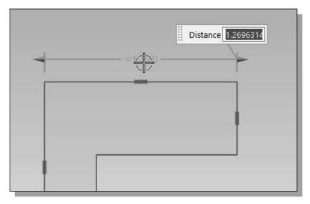
3. Enter **2.5** as the desired length of the line. (Press the **Enter** key once after you entered the new value.)
