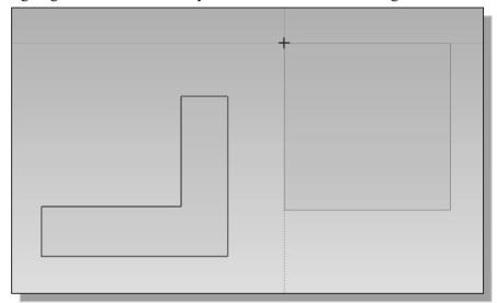
4. Create and modify the four size dimensions to describe the size of the sketch as shown. (Note that Siemens NX will maintain the right amount of dimensions to the sketch without over-constraining the sketch.)
