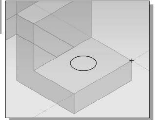
7. Select the **center point** of the circle and the **top edge** of the base to create the location dimension as shown. Set the dimension to **1.25** as shown.
