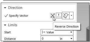
12. In the Direction option box, use the **Reverse Direction** icon to toggle the extrusion direction so that the extrusion cut through the bottom section of the model.
