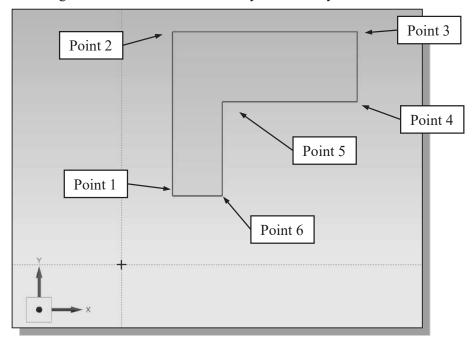
6. Inside the graphics window, click twice with the **middle-mouse-button (MB2)**, or press the [**Esc**] key twice, to end the Sketch Line command.
