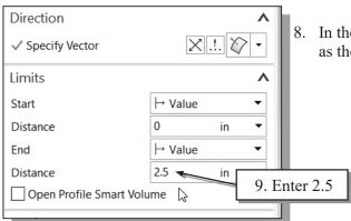
8. In the *Extrude* pop-up window, enter **2.5** as the extrusion distance.
