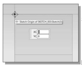
3. Use the **Profile** command and start the first line segment at the top left corner (the sketch Origin) as shown.
