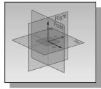
❖ The default sketch plane is aligned to the **Top - XY** plane of the Work Coordinate System.
