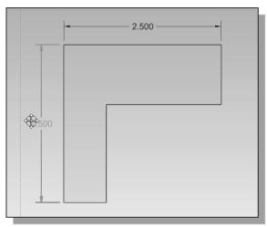
11. To reposition any of the dimensions, simply press and drag with the left-mouse-button (MB1) on the dimension as shown.
