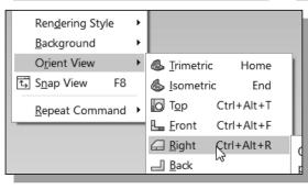
3. Inside the graphic window, right-click once to bring up the *Option menu*. Select **Right View** in the *Orient View List* to change the display to the right side view. (Note that the quick-key [Ctrl+Alt+R] can also be used to activate this command.)
