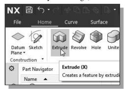
1. In the *Feature Toolbar* (toolbar next to the *Sketch* toolbar in the *Ribbon Bar*), select the **Extrude** icon as shown.
