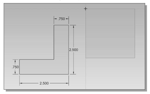
5. Create and modify the two location dimensions to **0.0**; this will align the position of the sketch relative to the top left corner of the solid model as shown.
