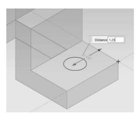
8. On your own, create and modify the size dimension and the other location dimension to 0.75, as shown in the figure. (Hint: there are two locational dimensions and one size dimension.)
