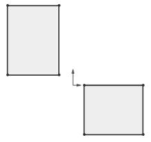
**1.2.** - Select the "Extruded Boss" command. Notice that we are not given a warning about having two separate bodies; it just works. Extrude the sketch any size that looks similar to the following image (dimensions are not important at this time) and click **OK** to finish. Making two or more extruded/revolved/swept features would work the same.
