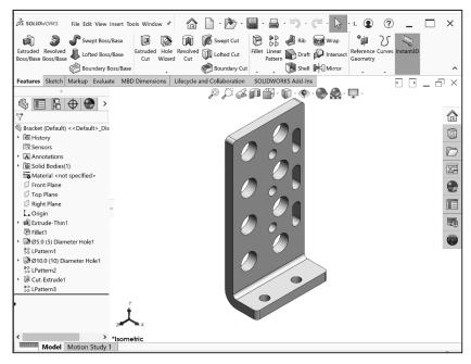
The FeatureManager design tree is located on the left side of the SOLIDWORKS Graphics window. The FeatureManager provides a summarized view of the active part, assembly, or drawing document. The tree displays the details on how the part, assembly or drawing document was created.
