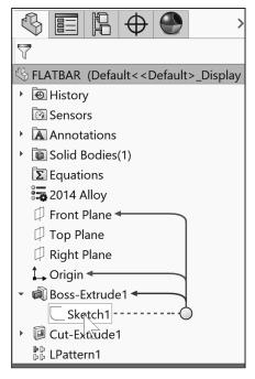
Use Dynamic reference visualization for a part, assembly and mates.
