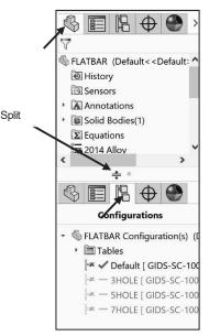
The ConfigurationManager tab is located to the right of the PropertyManager tab. Use the ConfigurationManager to create, select and view multiple configurations of parts and assemblies.
