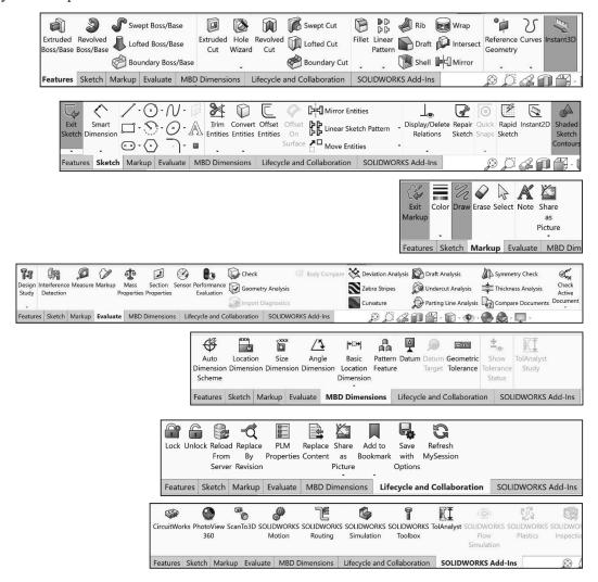
The SOLIDWORKS CommandManager is a Context-sensitive toolbar that automatically updates based on the toolbar you want to access. By default, it has toolbars embedded in it based on your active document type. The available tools are feature and document dependent.
