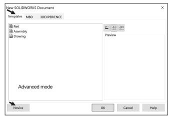
The Advanced mode remains selected for all new documents in the current SOLIDWORKS session. When you exit SOLIDWORKS, the Advanced mode setting is saved.
