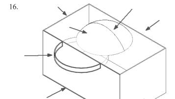
Select the four sides of the box, the outside arc of the cylinder and the two sides of the dome to place walls.
