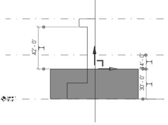
You can see how the dimensions are indicating the relative distances between the top face and the upper level, the bottom face, and another sketch.
