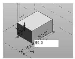
You will see two temporary dimensions. One dimension indicates the distance of the face to the opposite face (the length of the block). One dimension indicates the distance of the face to the closest work plane.
