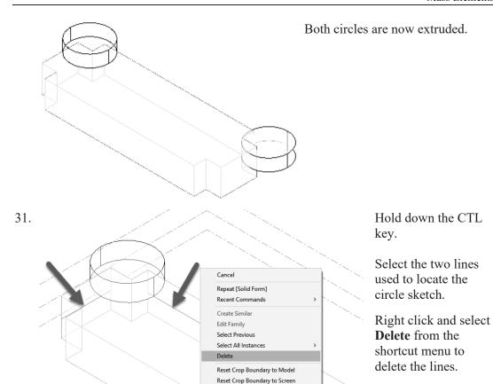
You can also click the Delete key on the keyboard or use the Delete tool on the Modify panel.
