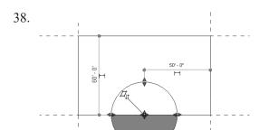
Place a cylinder at the midpoint of the bottom edge of the box.
