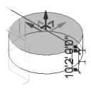
A preview of the extrusion will appear with the temporary dimension. You can edit the temporary dimension to modify the height of the extrusion.
