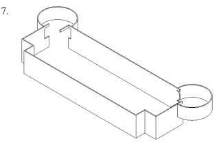
Select each wall and cylinder. The cylinder will be halved by the walls, so you will have to select each half.
