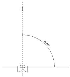
Select the center of the door as the start point of the mirror axis.
