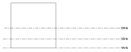
To adjust the horizontal position of the level lines, simply select the line and use the grip to extend or shorten it.
