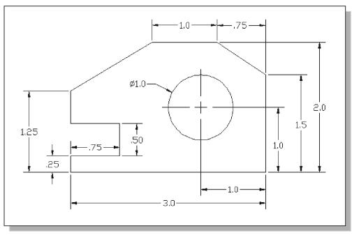
2. Spacer Plate (Thickness: .125)
