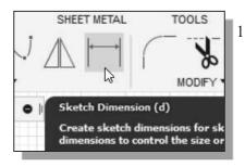
In the sketch toolbar, select the Sketch Dimension command as shown. The Sketch Dimension command is generally known as Smart Dimensioning in parametric modeling.
