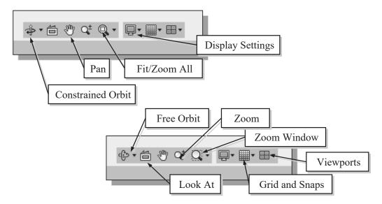
Orbit – In a part or assembly, adds an orbit symbol and cursor to the view. You can orbit the view planar to the screen around the center mark, around a horizontal or vertical axis, or around the X and Y axes.
