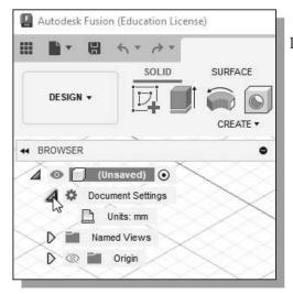
Click on the triangle icon next to the *Document Settings* option in the Browser area to show the default units as shown. Note the current units is set to the millimeter (mm) units as shown.
