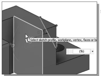
12. On your own, use the dynamic rotate function and select the back surface as shown.
