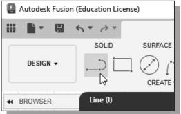
3. Select the **Line** command by clicking once with the **left-mouse-button** on the icon in the *Sketch* tab on the Ribbon.
