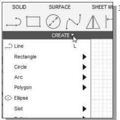
3. Click and press on the **Sketch** tab in the main *Ribbon* area to display the additional available sketching tools as shown. Also note the **Sketch Palette** panel is also activated with a variety of sketching options.
