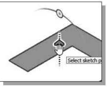
12. Move the cursor on top of the blue arrow on the selected region; notice the dashed line appears as shown. We can drag the arrow up or down, with the left mouse button, to set the extrusion distance and direction.
