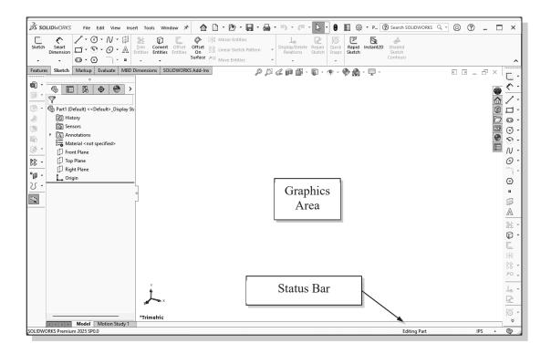
**IMPORTANT NOTE:** The SOLIDWORKS *CommandManager* provides a context-sensitive method for displaying the most commonly used toolbars. If the *CommandManager* is active, individual toolbars appear when the appropriate tab is selected. In the figure above, the *Sketch* tab is selected. Alternately, the *CommandManager* can be turned off and the individual toolbars displayed simultaneously, as shown on page 1-15. In this lesson, we will use the *CommandManager*.
