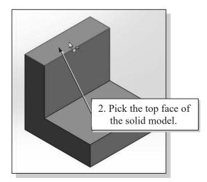
Note that the sketch plane is aligned to the selected face. SOLIDWORKS automatically establishes a local coordinate system, and records its location with respect to the part on which it was created.
