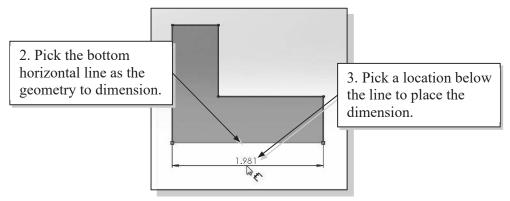
3. Move the graphics cursor below the selected line and left-click to place the dimension. (Note that the value displayed on your screen might be different than what is shown in the figure above.)
