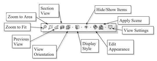
**Zoom to Fit** – Adjusts the view so that all items on the screen fit inside the graphics window.
