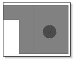
5. Create a circle of arbitrary size on the top face of the solid model as shown. Click once with the left-mouse-button to select the center of the circle, move and click again to set the radius. Press the [Esc] key once to end the Circle command.
