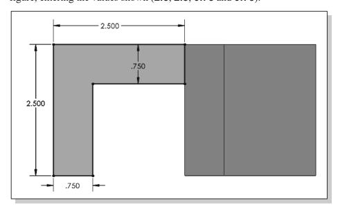
10. Click the **OK** icon in the *PropertyManager* as shown, or hit the [**Esc**] key once, to end the Smart Dimension command.
