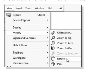
The Rotate View command allows us to rotate a part or assembly in the graphics window. Rotation can be around the center mark, free in all directions, or around a selected entity (vertex, edge, or face) on the model.
