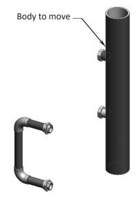
Click the **Constraints** button **Constraints** (at the lower left side of the tree) and click inside the **Mate Settings** section box to activate this option.
