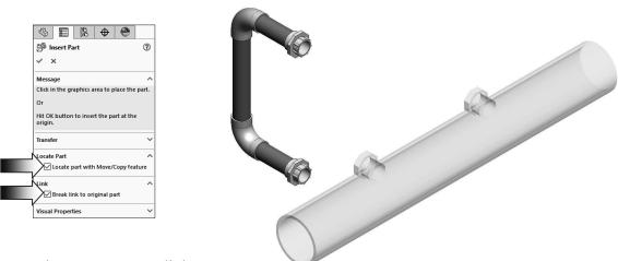
The **Locate part** dialog appears. We will use the Rotate options to reorient the large tube to the upright position.
