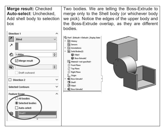
**1.8. -** The "Merge result" option works the same way with any feature that adds or removes material to the part, including revolved boss, sweep, loft, etc. Now we'll see how it works when material is removed. Delete the last Boss-Extrude feature and keep the sketch. When deleting the "Boss-Extrude," make sure the option "Delete absorbed features" is unchecked; this way the boss will be deleted, but the sketch will be left behind.
