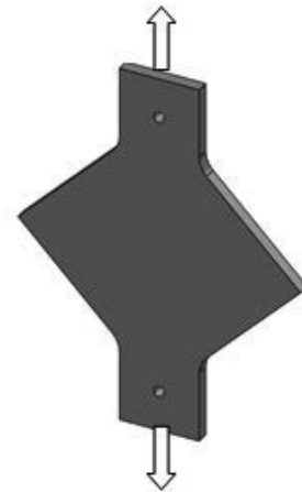
Figure 37 - Model subject to “equal” but opposite forces.
