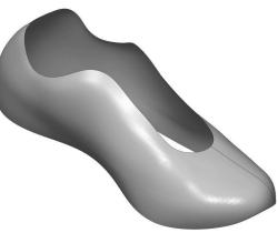
Surfaces can be used as reference geometry in order to assist with the construction of a model. The surfaces will then be moved into a Surface Bodies folder and become hidden when the model is complete.
