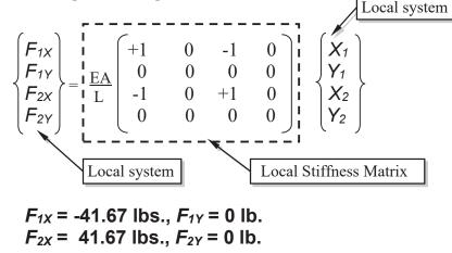
Therefore, the normal stress developed in *Element A* can be calculated as (41.67/0.049)=**850 psi**.
