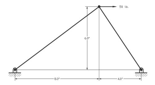
Material: Steel rod, diameter <sup>1</sup>/<sub>4</sub> in.
