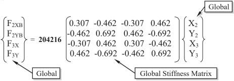
Now we are ready to assemble the overall global stiffness matrix of the structure.
