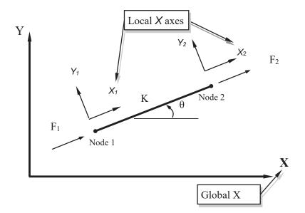
The force-displacement equations expressed in terms of components in the local XY coordinate system:
