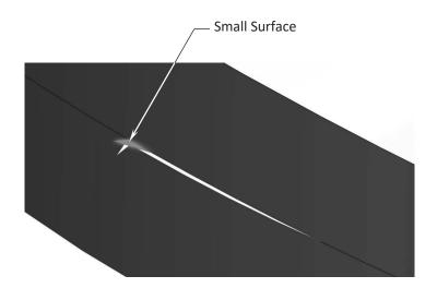
On the <u>right end</u> of the model, there is also a small triangular surface that did not get trimmed correctly.
