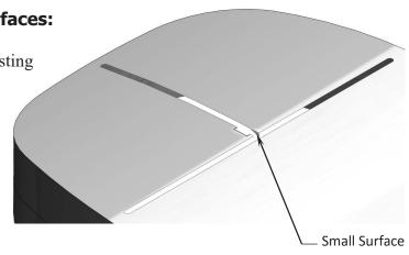
On the <u>left side</u> of the model, there is a gap and a small triangular surface in this area.
