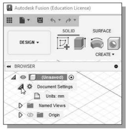
1. Click on the triangle icon next to the **Document Settings** option in the Browser area to show the default units as shown. Note the current units is set to the millimeter (mm) units as shown.
