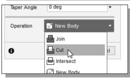
12. Select the **CUT** option in the *feature option* list to set the extrusion operation to *Cut*.
