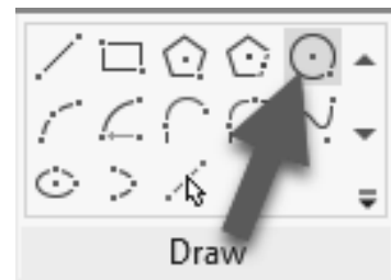
FIGURE 3-1.16 Detail Line shapes
