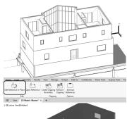
Use the MOVE tool to adjust the XREF position to align one of the building corner's with the existing model.
