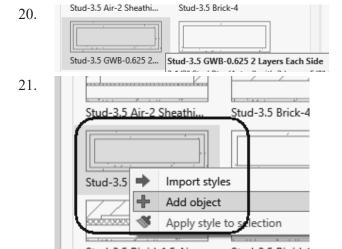
Locate the Stud -3.5 GWB-0.625 2 Layers Each Side wall style.
