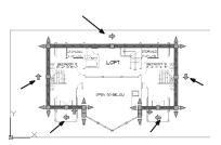
Verify that all the walls are oriented with the exterior side on the outside of the building.
