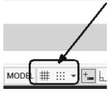
Toggle off the Grid and Snap to Grid.
