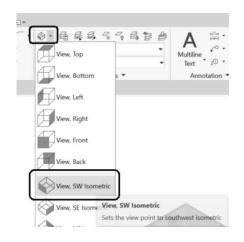
On the Home ribbon: Switch to a **SW Isometric view**.
