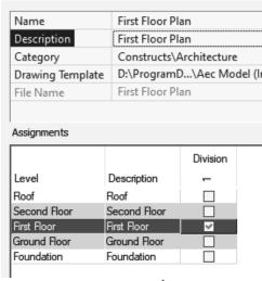
Assign **First Floor Plan** to the Name.
