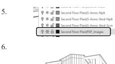
Locate the **Second Floor Plan**|**PDF Image** layer in the layer drop-down list. Freeze the layer.
