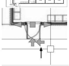
If required, select the placed door. Use the arrows to flip the door so it is oriented correctly.
