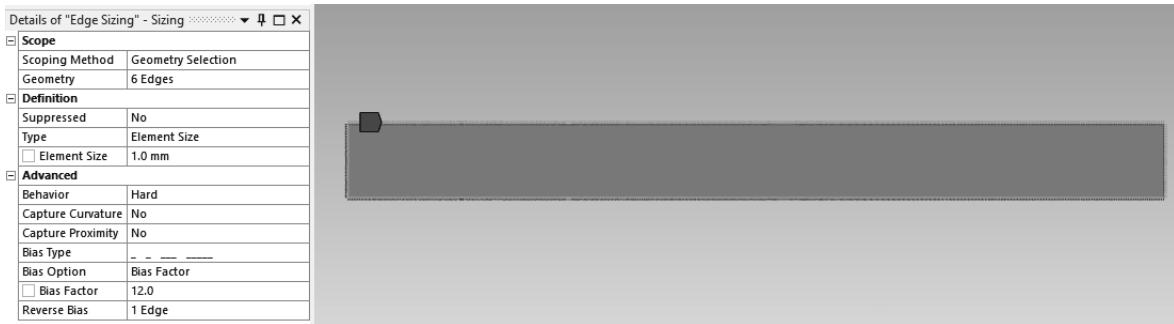
Figure 2.5g) Details of edge sizing for three of the horizontal edges and the vertical edges
