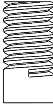
Cut - Thread removed from Major Diameter
