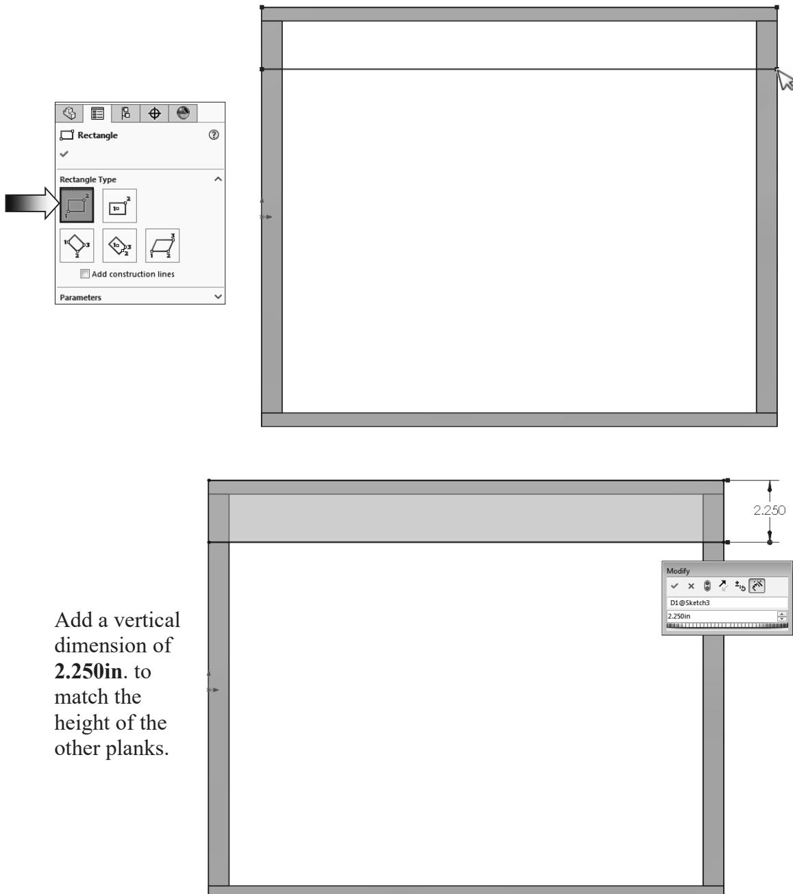
Change to the **Isometric** view (Control+7) before extruding the sketch.
