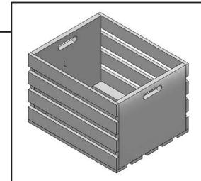
A general rule to keep in mind is that one part, multibody or not, should represent one part number in a Bill of Materials. A multibody part consists of multiple solid bodies that are not dynamic. If dynamic motion among bodies is needed it should be done in an assembly instead. Tools such as Move Component, Dynamic Clearance, and Collision Detection are available only with assembly documents.
