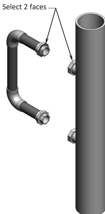
A **Coincident** mate is created. The large tube moves forward and touches the fixed body. Click **Add** to accept the mate.
