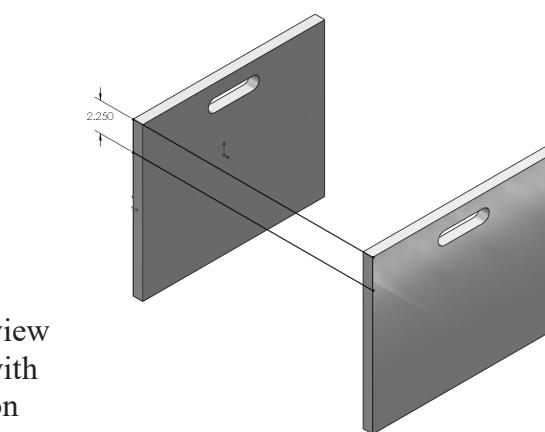
Change to the **Isometric** view (Control+7); it will help with seeing the extrude direction more clearly in the next step.
