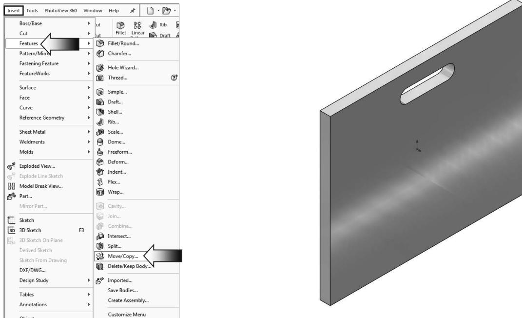
To add commands to a toolbar: Select Tools / Customize / Commands / Features and drag/drop the Move/Copy command to your Features tool tab.
