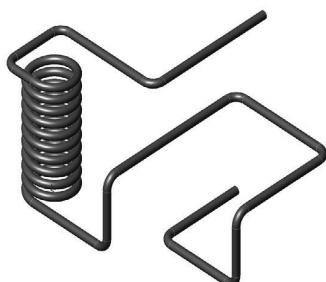
A 3D sketch usually consists of lines and arcs in series and Splines. You can use a 3D sketch as a sweep path, as a guide curve for a loft or sweep, a centerline for a loft, or as one of the key entities in a routing system.
