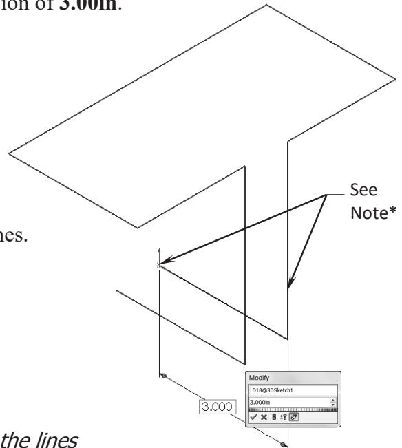
**Note:** To make the dimensions parallel to the lines as shown, select the line and an endpoint instead of selecting the two endpoints; the dimension will be parallel to the line.
