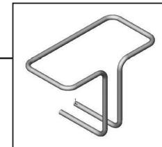
SOLIDWORKS has 3D sketch capabilities. A 3D sketch consists of lines and arcs in series and splines. You can use a 3D sketch as a sweep path, as a guide curve for a loft or sweep, a centerline for a loft, or as one of the key entities in a piping system. Geometric relations can also be added to 3D Sketches.
