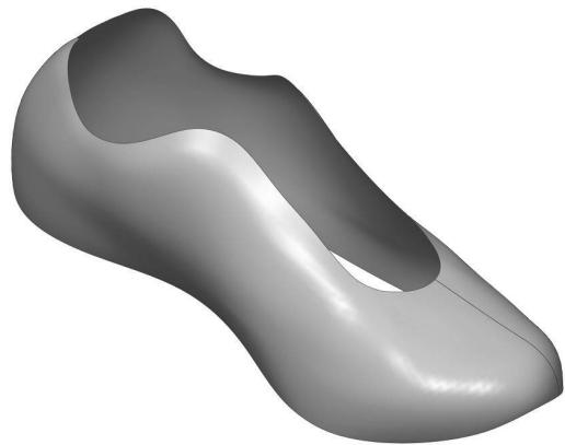
Surfaces can be used as reference geometry in order to assist with the construction of a model. The surfaces will then be moved into a Surface Bodies folder and become hidden when the model is complete.
