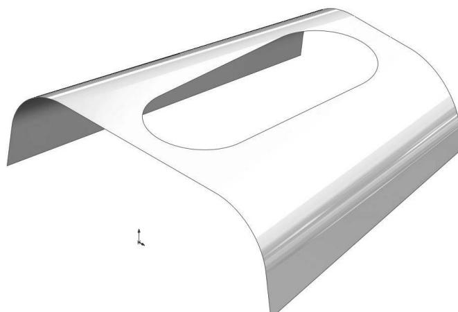
For Surface Split Option, select: **Natural** to match the existing curvature of the surface model.
