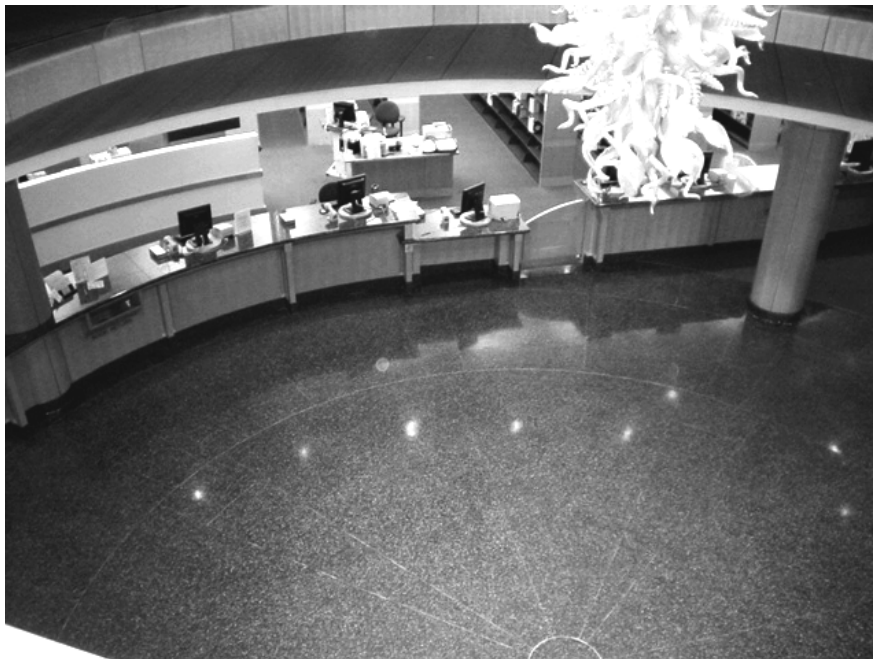
CHECKOUT COUNTER EXAMPLE Second floor view showing gate and accessible checkout area with lower countertop.
