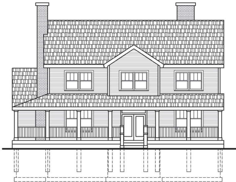
Exterior Elevation created in Chapter 5, utilizing blocks, hatching, lineweights and line types.
