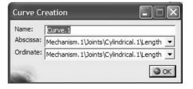
For Abscissa, select Mechanism.1\Joints\Cylindrical.2\LengthAngle For Ordinate, select Speed-Acceleration.2\LinearSpeed
